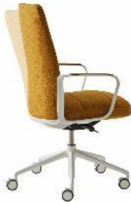
Synchronized mechanism. Swivel base on casters. Seat height adjustment with gas lift. Synchronized tilt movement of the seat and back. Four locking positions. Tension adjustment to user weight.
